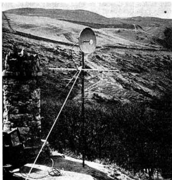
Looking out across the Irish Sea to the Isle of Man is the 23cm dish of GW3XAD/P in readiness for the believed-first GW to GD contact on this band. At the other end was GD3TPF/P
